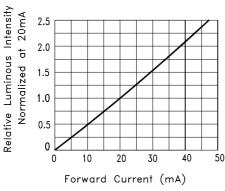
Fig.4 Relative Luminous Intensity vs. Forward Current
